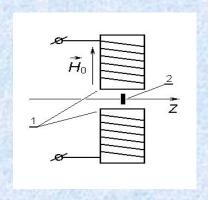
1 - solenoid;  $2 - \text{sample (FeBO}_3),$  $4 \times 3.5 \times 0.25 \text{ mm}.$
