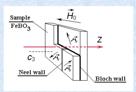
This figure shows the magnetic structure of the sample. One can see the Neel wall and the Bloch wall. The arrows indicate the magnetization M<sub>s</sub> within the domains.
